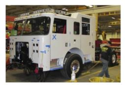
The cab of the ladder truck during the manufacturing process.
