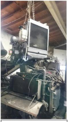
Pictured above, the old motor being removed from the street sweeper. That part was on a platform with many other parts attached, including the radiator (the large black part in the foreground). DPW personnel successfully detached and removed the old motor, attached the new motor and installed it back in the sweeper.
